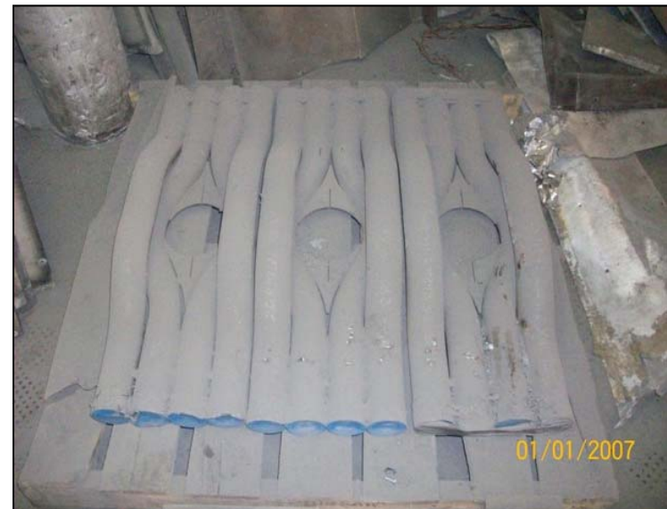
Boiler Tube Insert for SNCR System
